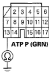
Fig. 421: Checking Continuity Between PCM Connector Terminal D13 And Body Ground Courtesy of AMERICAN HONDA MOTOR CO., INC.
